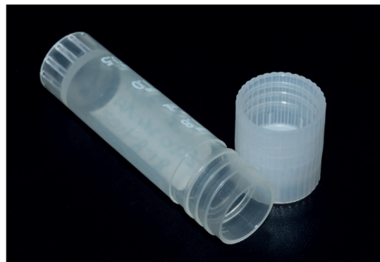
2ml screw cap storage tubes, with an O-ring to prevent leakage, used to store the tissue samples.
