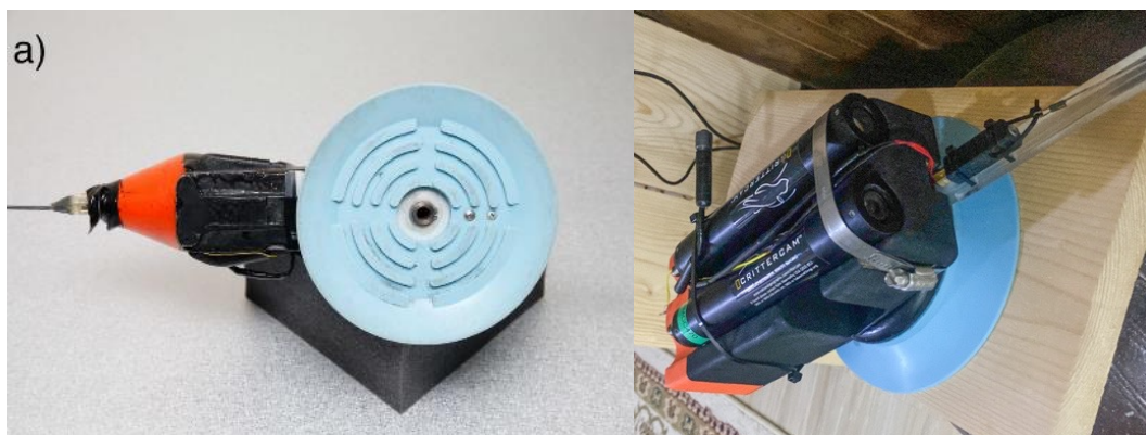
Figure 8: The old (a) and new (b) designs of the National Geographic Society Crittercam systems.
